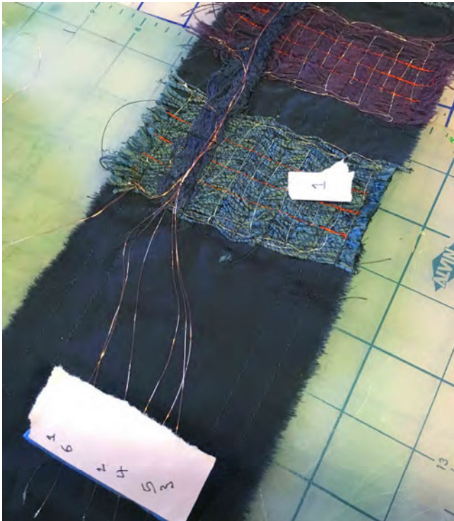
Figure 7: Incorporating the conductive touch points and connecting the enameled lead wires.
