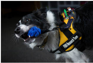
Figure 3: Alerting using tug sensor.
